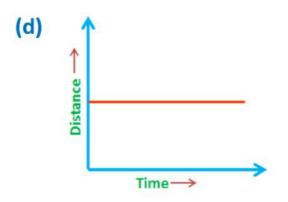
**About:** In this graph, an object is at rest as the distance remains constant with increase in time.
