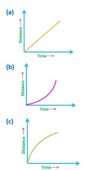
**About:** In this graph, the object covers equal distances in equal intervals of time and so its speed is uniform.
