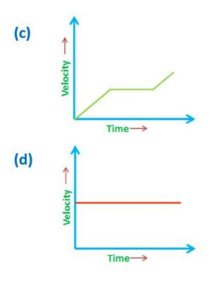
**About:** In this graph, the velocity of the object is increasing non - uniformly.
