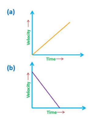
**About:** In this graph, the velocity of the object is increasing by equal amounts in equal intervals of time.
